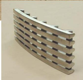
Wedge shaped wire construction welds stainless steel rods in precise alignment to achieve the best combination of flow rate and strength.
